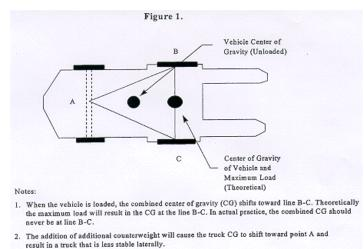
A-4.2. When the vehicle's line of action, or load center, falls within the stability triangle, the vehicle is stable and will not tip over. However, when the vehicle's line of action or the vehicle/ load combination falls outside the stability triangle, the vehicle is unstable and may tip over. (See Figure 2.)
