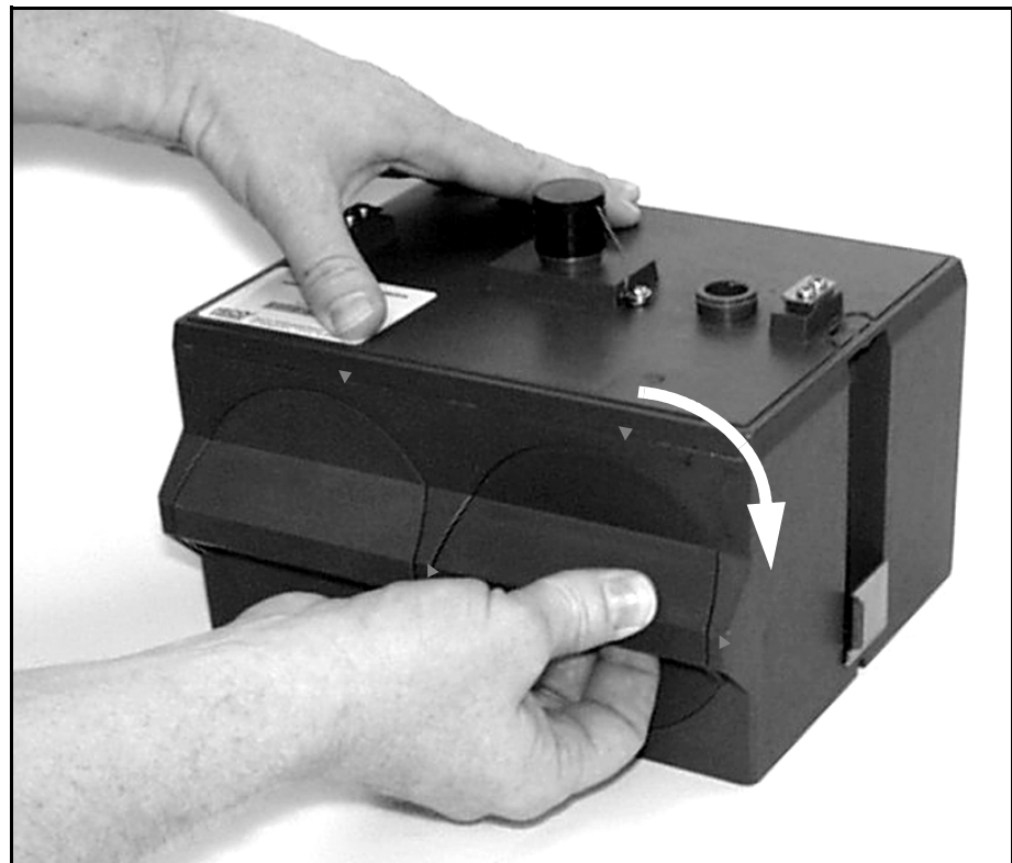
Figure 1-15 Battery Module - closing the door
