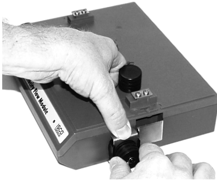
Figure 1-10 Flow Module - preparing the sensor connectors
