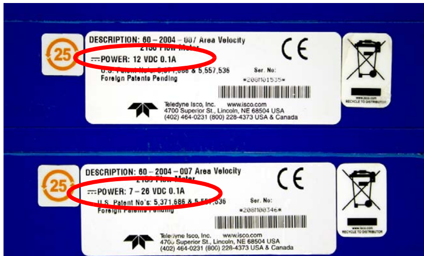
Figure 2-1 Identifying the 2150 voltage specification
