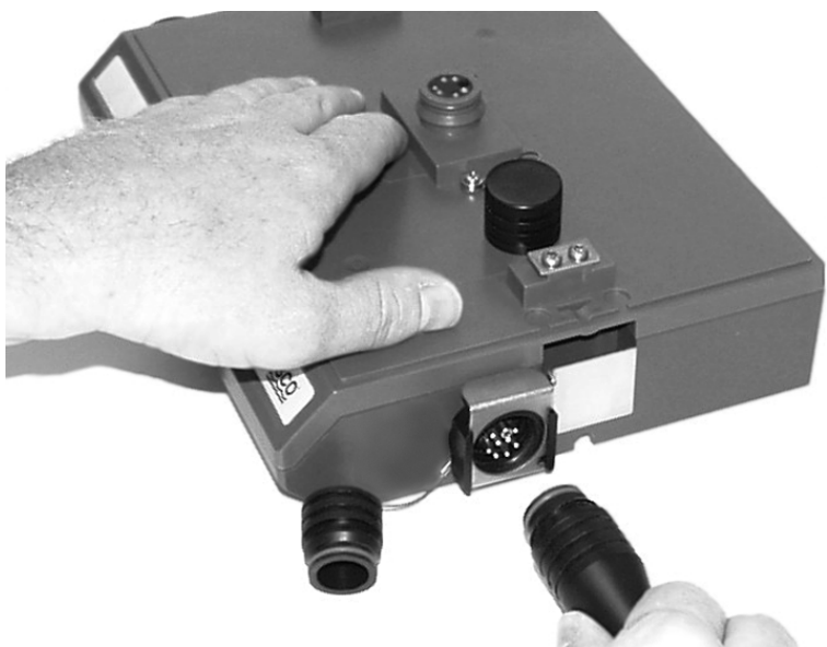
Figure 1-10 Flow Module - preparing the sensor connectors
