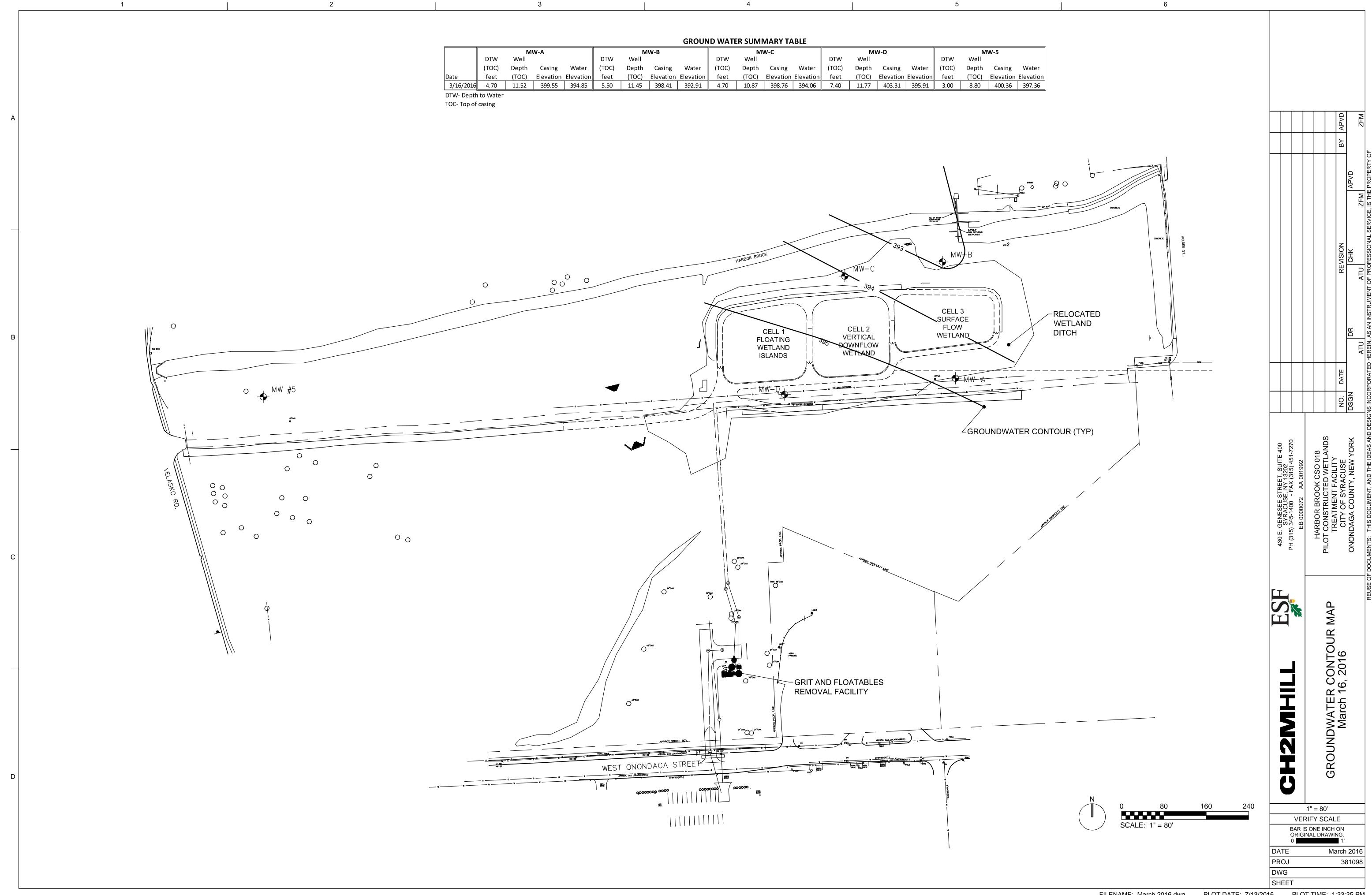
**GROUND WATER SUMMARY TABLE** MW-C DTW DTW Well | Casing | C DTW- Depth to Water TOC- Top of casing MW-BCELL 3 SURFACE \_\_RELOCATED WETLAND FLOW WETLAND CELL 2 VERTICAL DOWNFLOW CELL 1 DITCH FLOATING WETLAND WETLAND ISLANDS O MW #5 -GROUNDWATER CONTOUR (TYP) 0 0 0 0 00 -GRIT AND FLOATABLES REMOVAL FACILITY WEST ONONDAGA STREET SCALE: 1" = 80' VERIFY SCALE BAR IS ONE INCH ON ORIGINAL DRAWING.
