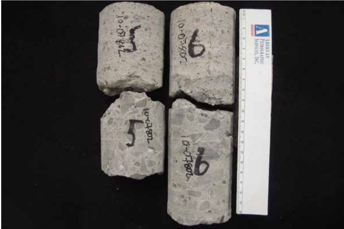
SAMPLE ID: 5 and 6 DESCRIPTION: Overall view of concrete core samples as received.
