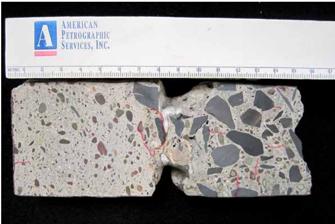
SAMPLE ID: 5 DESCRIPTION: Overall view of a cut and polished cross section of the sample. The outer concrete is on the left side and inner concrete is on the right side of the photo. Microcracking was mapped in red ink.
