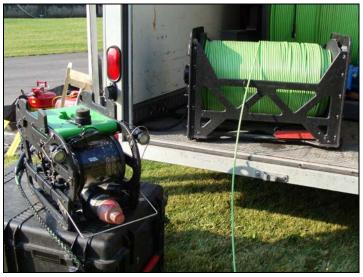
Figure 2: LBV ROV Prior to Deployment
